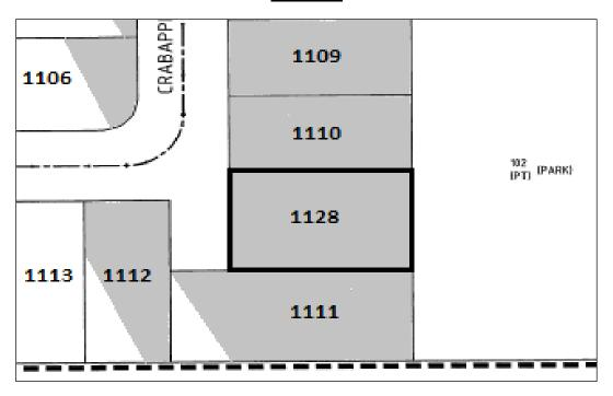
Approximate lateral extent and maximum depth of controlled filling to 2.0m. Level 1 Certification is limited to within this area.
