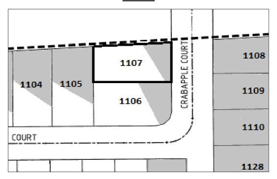
Approximate lateral extent and maximum depth of controlled filling to 0.3m. Level 1 Certification is limited to within this area.
