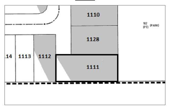
Approximate lateral extent and maximum depth of controlled filling to 1.5m. Level 1 Certification is limited to within this area.
