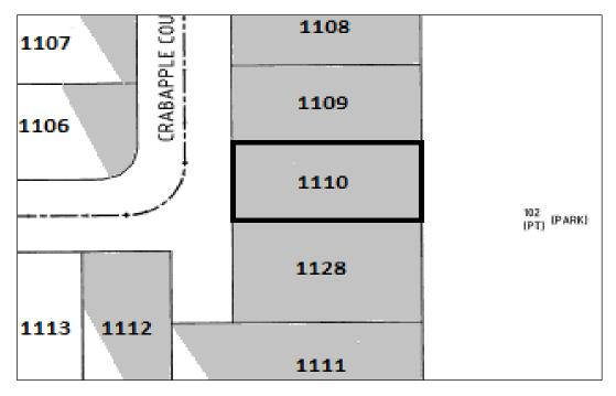
Approximate lateral extent and maximum depth of controlled filling to 2.2m. Level 1 Certification is limited to within this area.
