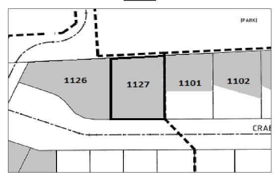
Approximate lateral extent and maximum depth of controlled filling to 0.5m. Level 1 Certification is limited to within this area.
