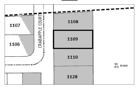
Approximate lateral extent and maximum depth of controlled filling to 2.3m. Level 1 Certification is limited to within this area.
